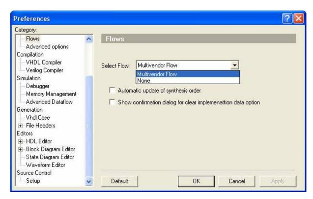
Selecting the **Multivendor Flow** will give you the option to choose the desired Synthesis Tool and Implementation Tool, Xilinx ISE later in the **Flow Settings** window. But first, you must open
