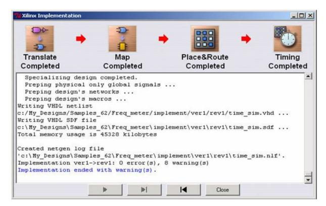
When implementation is completed, a subfolder labeled **Timing** is added to the Active-HDL Design Browser window. This folder contains all the necessary files to perform timing simulation (VHDL or Verilog) including the SDF file.
