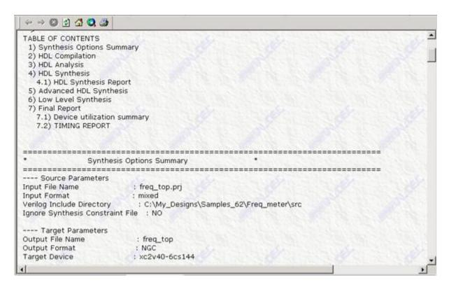
When synthesis is successfully completed, a check mark is displayed next to the button in the flow menu. The file created after synthesis using Xilinx's XST is in .ngc file format. Below, is a list of the other marks that might appear in the flow chart during Synthesis and Implementation:
