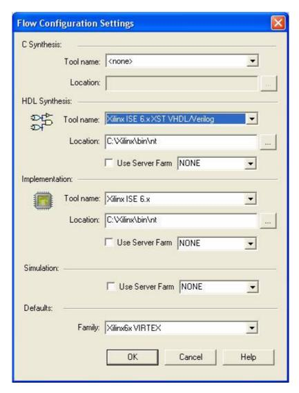
After selecting the desired Synthesis and Implementation Tool, the option to use Server Farm for synthesis and implementation is automatically added. Additionally, you can also select the option to use Server Farm for Simulation. In the lower part of the window, you can select the Family of Xilinx devices.
