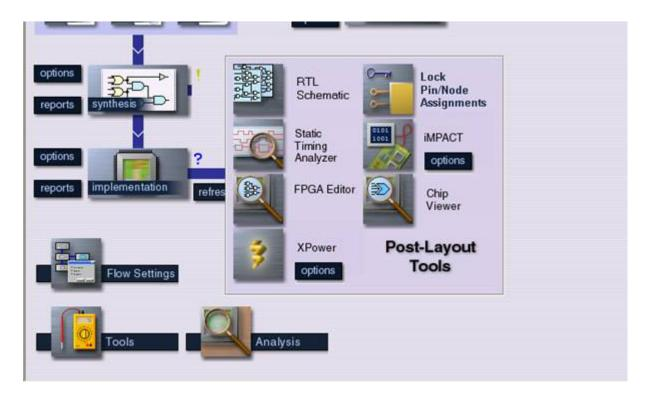
Note that the settings for timing simulation must be configured first, you can do this by clicking on its corresponding **options** button. For a more detailed description of the timing simulation procedures, refer to app note titled "Timing Simulation in Active-HDL".
