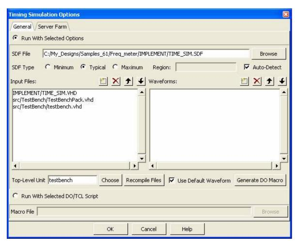
Choose the .SDF file and .vhd file generated after implementation as chosen in the diagram. Also choose a top-level unit. You can also choose the SDF type to be minimal, typical or maximum. After making your selections, click on the timing simulation icon in the design flow manager. Active-HDL will start compiling the design files and after simulation has been initialized you should be seeing the following message in your Active-HDL console:
